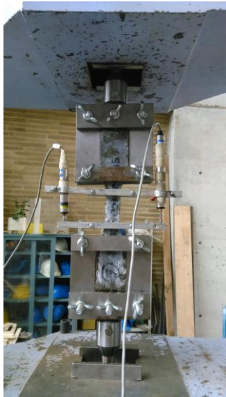
Fig. 2. Direct tensile test set-up (left) and strain-stress behavior of the optimized UHPFRC (right).
