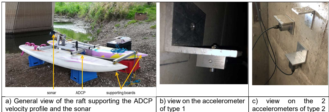
Figure 5. Details of the instrumentation set-ups.
