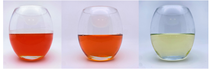
Fig. 2. Crude and refined oils from DHA ORIGINS ® 550 range (Fermentalg). From a single crude oil, different refined oils in term of color could be obtained. (a) crude algal oil; (b) refined orange oil (DHA ORIGINS ® 550-O); (c) refined decoloured oil (DHA ORIGINS ® 550-Y).
