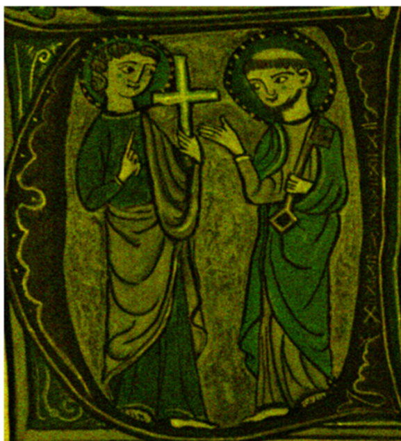
Figure 11 UV False color of the facsimile at 610 nm (R =590 nm, G =610 nm & B =800 nm). Thanks to spectrofluorimetric study, the imagery under UV obtained with the hyperspectral camera allows us to map the cinnabar which emits fluorescence at 610 nm.
