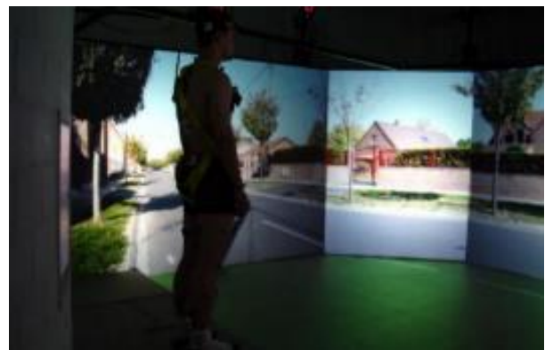
Figure 19 Simulator-based system for studying street-crossing. Source: Julie Delzenne's doctoral thesis, 2013, UPHF, p. 147, http://www.theses.fr/2013VALE0031 (accessed 03/05/2021)
