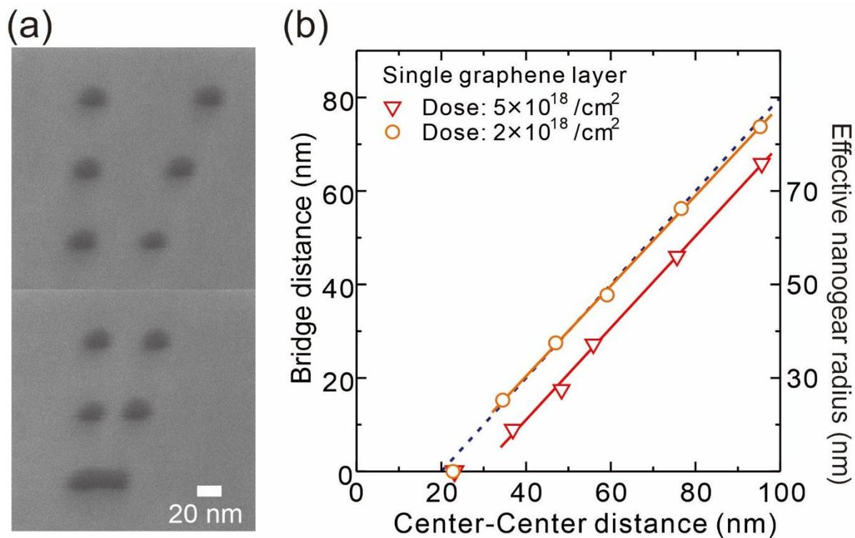
**Figure 5.** (a) The low dose HIM image of a series of two rectangular patterns on a graphene monolayer suspended on a TEM grid. (b) The relationship between the center-center distance and bridge distance for this suspended graphene monolayer using different He<sup>+</sup> doses.
