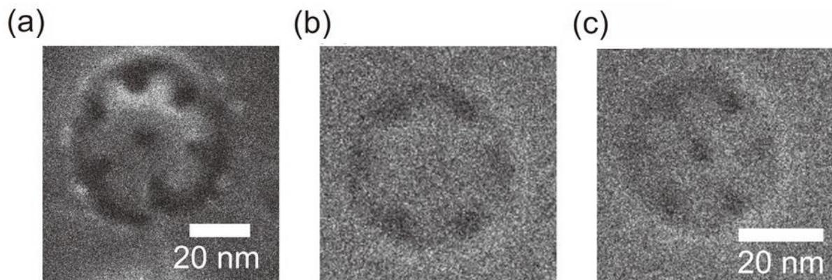
**Figure 3.** HIM images of a nanogear sculptured using a  $\text{He}^+$  ion focused beam irradiation in (a) a 20 nm in thickness gold layer ( $1.5 \times 10^{19}$  ions/cm<sup>2</sup>), (b) a graphene multilayer (4 - 5 layers thickness) before ( $2 \times 10^{18}$  ions/cm<sup>2</sup>) and (c) after making the center hole ( $1 \times 10^{20}$  ions/cm<sup>2</sup>).
