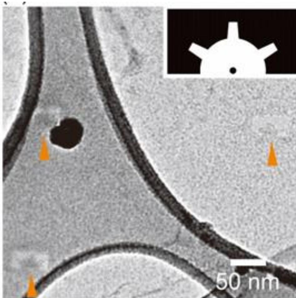
**Figure 6.** The TEM image of nanopatterns (marked by orange arrows) sculptured by focused  $\text{He}^+$  ion beam in a single suspended graphene monolayer on a TEM grid. Inset: Nanopattern where black area is scanned by the  $\text{He}^+$  focused ion beam. Note that the sample was taken out in air after its Orion  $\text{He}^+$  ion milling and then moved on the stage of an ultra-high vacuum TEM (JEOL, JEM-2100F, 200 keV).
