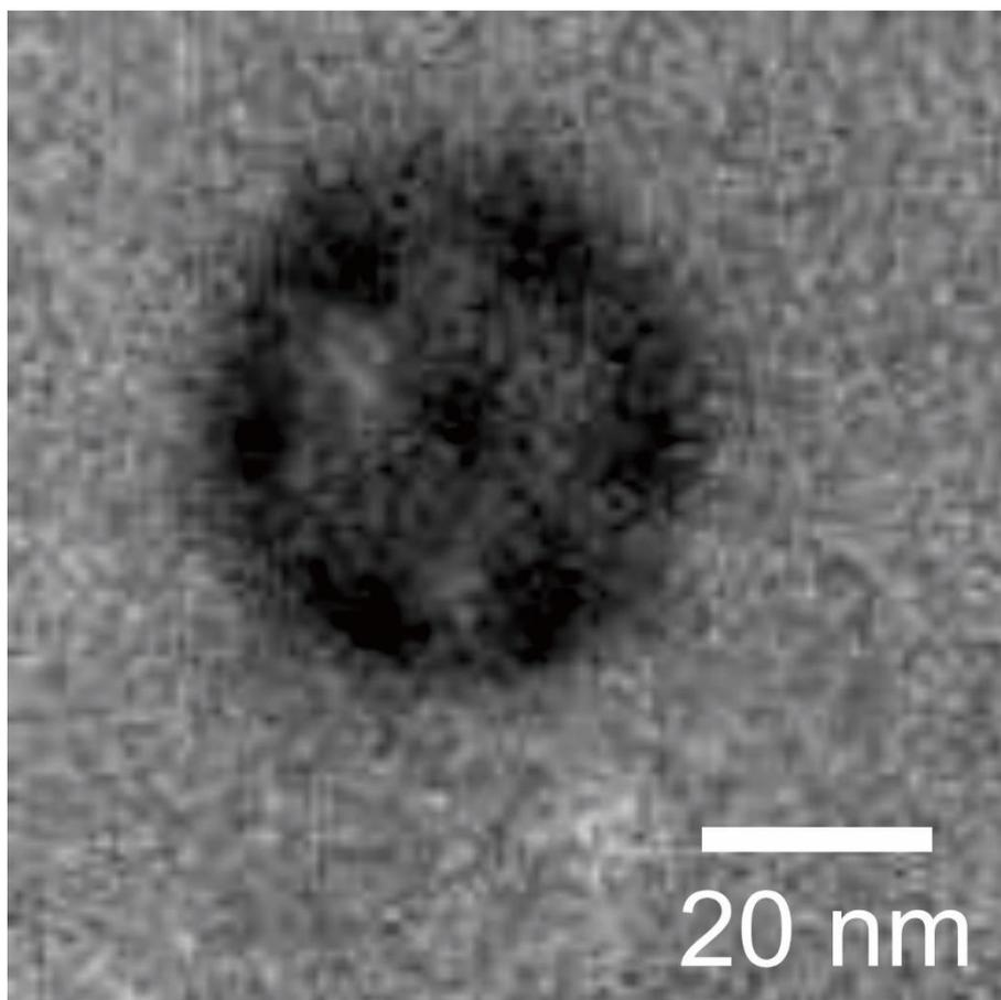
**Figure 4.** HIM images of a single nanogear milled in a graphene monolayer with also its central hole for the rotation axle by using a dose of  $9 \times 10^{18}$  ions/cm<sup>2</sup>.
