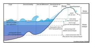
Figure 3. Forcings acting during a marine flood (Courtesy : Nicolae-Lerma)
