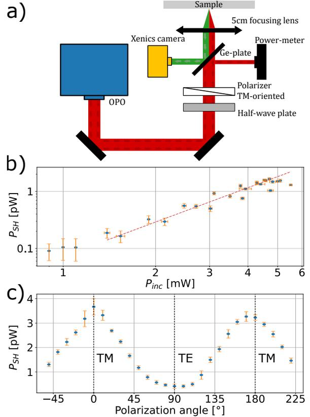
**Fig. 4.** a) Schematic of the non linear characterisation set-up b) The measured second-harmonic signal power as a function of the incident pump power. The red line is a least-square regression corresponding to the following mathematical expression:  $\log(P_{SH}) = 2 \cdot \log(P_{inc}) - 1.138$ . c) The second-harmonic signal power as a function of the incident pump polarization angle.
