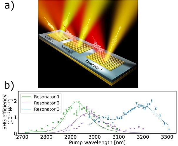
**Fig. 5.** a) An illustration of the concept of a broad-band SHG nanodevice. b) Measured and simulated SHG conversion efficiency spectra obtained for  $w_1 = 295$  nm,  $w_2 = 350$  nm,  $d = 1215$  nm (blue line),  $w_1 = 280$  nm,  $w_2 = 365$  nm,  $d = 1015$  nm (purple line) and the structure from Fig. 1 c) (green line). All three resonators have been designed using the same thicknesses of the golden nanoantennas  $t = 60$  nm and the GaAs nonlinear layer  $h = 142$  nm.
