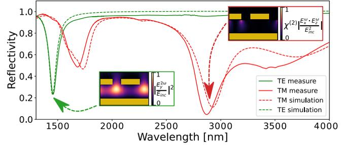
**Fig. 3.** Simulated and measured linear reflectivities of the structure. In inset the simulated normalized field component amplitudes in the structure at pump ( $\lambda_{\text{pump}} = 2.93$   $\mu\text{m}$ ) and signal ( $\lambda_{\text{signal}} = 1.46$   $\mu\text{m}$ ) resonances.
