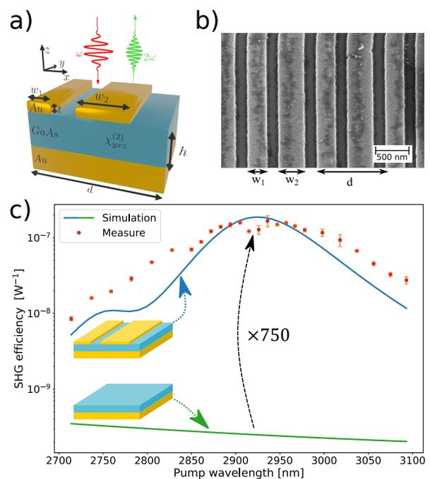
**Fig. 1.** a) Schematic representation of the resonator. b) A scanning microscope image of the sample. c) The measured and simulated SHG efficiency spectra of the coupled resonator nanostructure. The resulting efficiency is 750 times higher compared to a non-engineered equivalent GaAs layer reference.
