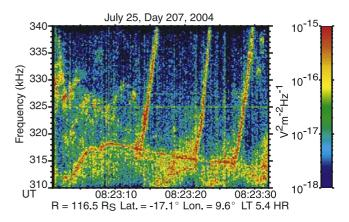
**Figure 3.** A remarkable frequency-time spectrogram centered at 325 kHz showing a series of rapidly rising tones ( $\sim$ 10 kHz/s) evidently triggered by a narrowband tone with a slight negative drift.
