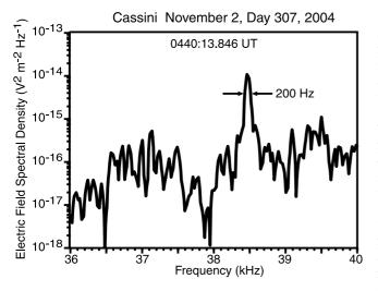
**Figure 2.** Detail of a single spectrum showing the narrowband feature at 38.5 kHz seen in Figure 1c. The spectral resolution is about 25 Hz, so the narrowband emission is resolved and has a bandwidth of about 200 Hz.
