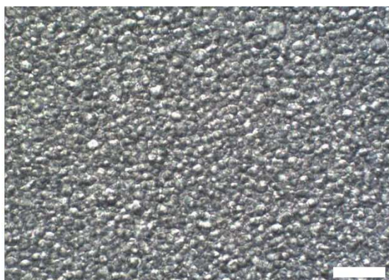
Figure 11. Optical micrograph of the final emulsion (sample #10) containing 25 parts of the oil mixture ( T = 25\text{ }^{\circ}\text{C} ; Hoffman modulation contrast; scale bar 20\text{ }\mu\text{m} ).
