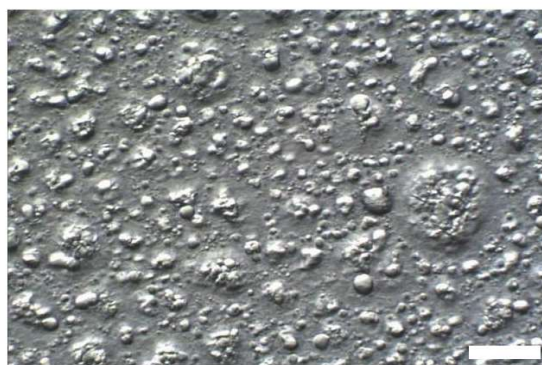
Figure 7. Optical micrograph of sample #6 containing two parts of oil added to the system consisting of emulsifier/consistency enhancer/water ( T = 25\text{ }^{\circ}\text{C} ; Hoffman modulation contrast; scale bar 20\text{ }\mu\text{m} ).
