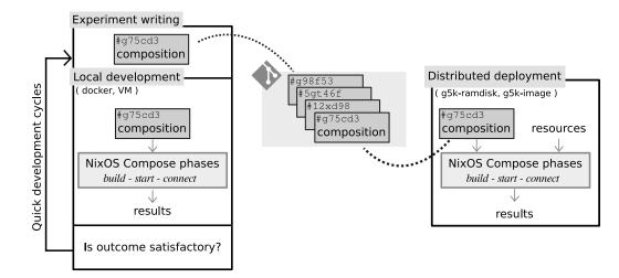
Fig. 4. Workflow of *NixOS Compose*. Local development of the environment is done using light and fast development with containers and virtual machines. Once the description of the environment (composition) has been tested, deployments on a distributed platform can be done with the **exact same interface**.
