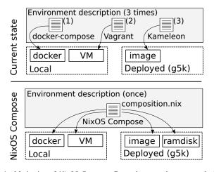
Fig. 1. Motivation of *NixOS Compose*. Currently, to produce a reproducible environment for each platform, users must maintain a description file for each target platform. We want *NixOS Compose* to only use a **single description** file (called a composition) that can build reproducible distributed environments and deploy them to **several platforms**.
