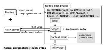
Fig. 5. Mechanism for the nodes to get the deployment information. For a small number of nodes, the information is passed via the kernel parameters. For a higher number of nodes, this is not possible due to the size limit on the kernel parameters (4096 bytes). In this case *NixOS Compose* starts a light HTTP server on the frontend and passes its URL to the nodes via the kernel parameters. The nodes then query this server to retrieve the deployment information.
