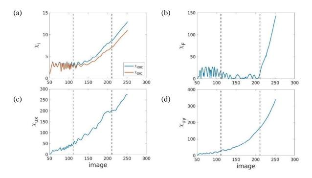
*Figure 14 - Instantaneous image (a), force (b) and displacement (c-d) residuals as functions of the image number. The dashed vertical lines depict the transitions between the elastic, elastoplastic and damage regimes.*
