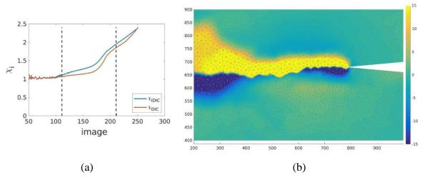
Figure 18 - (a) Instantaneous image residual as a function of image number. The dashed vertical lines depict the transitions between elastic, elastoplastic and damage regimes.
