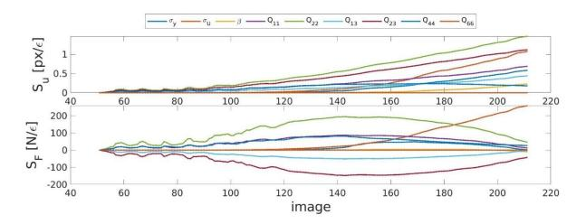
Figure 5 - Global displacement [px/perturbation factor] and force [N/perturbation factor] sensitivities as functions of image number for all elastoplastic parameters using an orthotropic elastoplastic model.
