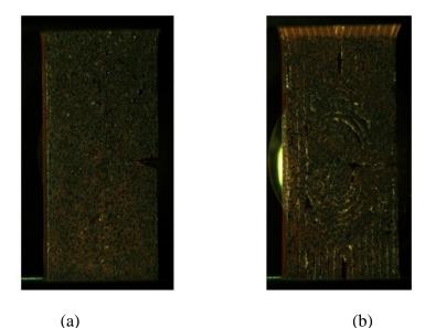
*Figure 22 - Reference pictures of (a) the specimen with* ± 45° *orientation, and (b) optimized orientation. The width of the samples was equal to 8 mm*
