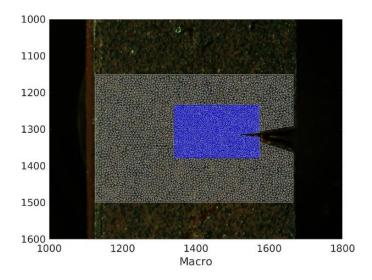
Figure 15 - Meshes used in mesoscopic (blue, 10px-elements at the mesoscale) and macroscopic (white, 5pxelements of the macroscale) DIC analyses. Scale: 1 macroscopic  $px \equiv 3.82$  mesoscopic px.
