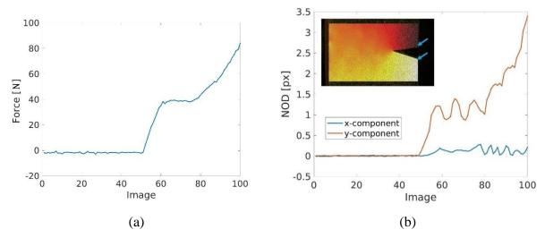
Figure 8 - (a) Force as a function of image number illustrating measurement fluctuations before image 51, and load application thereafter (beginning of the experiment).
