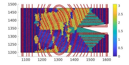
Figure 19 - Mesh for the optimized SENT specimen showing the different material orientations [rad]. The printing contours (red lines) are overlaid, element length = 5px.
