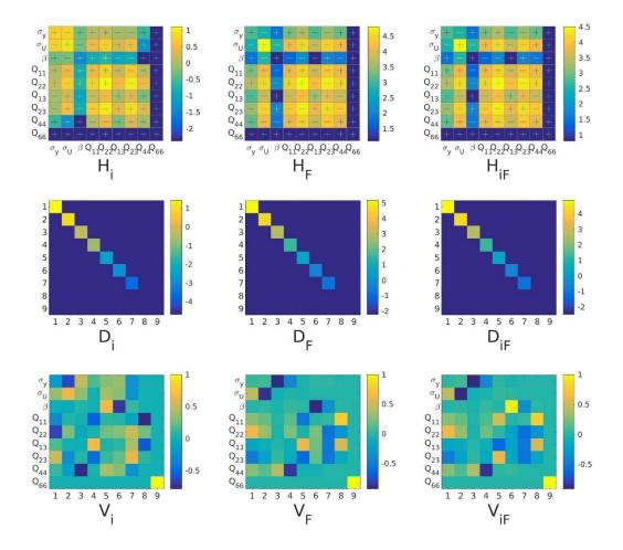
Figure 6 - Absolute image (left column), force (middle column) and image-force (right column) Hessians of the initial estimation (log<sub>10</sub> scale, first row), with their eigenvalues (log<sub>10</sub> scale, second row) and the corresponding eigenvectors (third row).
