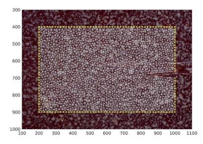
Figure 16 - Mesoscale mesh in white and boundary nodes in yellow, element length = 10 px.
