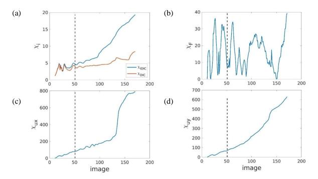
*Figure 21 - Instantaneous image (a), force (b) and displacement (c-d) residuals as functions of image number. The dashed vertical lines depict the transitions between the elastic and elastoplastic regimes.*
