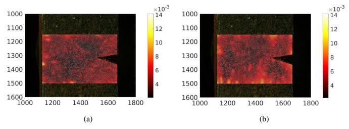
*Figure 7 - Horizontal (a) and vertical (b) components of the standard displacement uncertainty fields [px], element length = 5px.*
