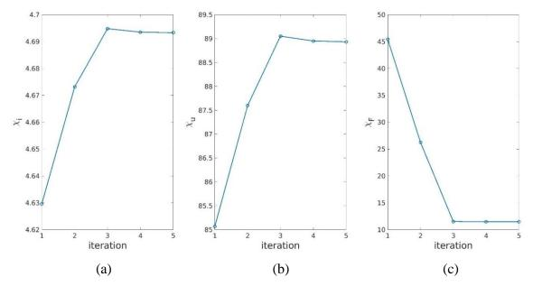
Figure 10 - Change of image (a), displacement (b) and force (c) residuals as functions of iteration number.
