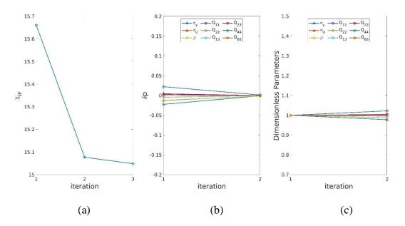
Figure 20 - Changes in total residuals (a), corrections on dimensionless parameters (b), and dimensionless parameters (c) as functions of iteration number showing the convergence of I-DIC using an orthotropic elastoplastic model.
