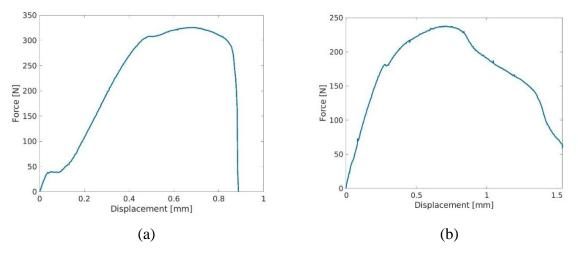
Figure 3 - Force-displacement plots of (a)  $\pm 45^{\circ}$  (b) optimized SENT samples. A higher maximum force is observed in the  $\pm 45^{\circ}$  case, and larger maximum displacement in the optimized configuration.
