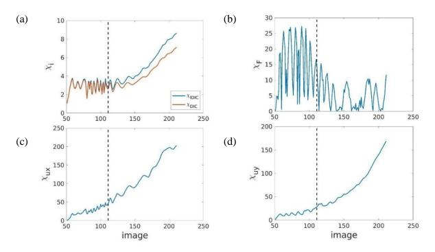
*Figure 11 - Instantaneous image (a), force (b) and displacement (c-d) residuals as functions of image number. The dashed vertical lines depict the end of the elastic regime and the transition to the elastoplastic regime.*
