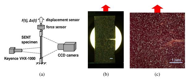
Figure 2 - (a) Schematic drawing of the experimental setup. (b) Macroscopic image acquired with the telecentric length, and (c) corresponding mesoscopic obtained with the Keyence VHX 1000. The red arrows indicate the tensile direction and the scale have the same value: 1 mm.
