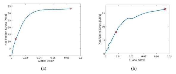
Figure 4 - Net section stress-strain plots for the  $\pm 45^{\circ}$  (a) and optimized (b) SENT specimens. The red circles depict the end of elastic and elastoplastic phases.
