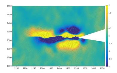
Figure 13 - Difference of y-displacement fields ( $y_{FEM}$  -  $y_{DIC}$ ) indicating crack propagation at maximum load (image 251), element length = 5px.
