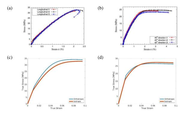
Figure 23 - Stress/strain plots of tensile experiments with (a) longitudinal and (b)  $45^{\circ}$ -oriented filaments [42]. True stress vs. true strain of tensile simulations using the calibrated parameters of the (c) optimized specimen and (d)  $\pm 45^{\circ}$  specimen. The small difference between the responses using isotropic or orthotropic elasticity validates the conclusion of weak elastic anisotropy.
