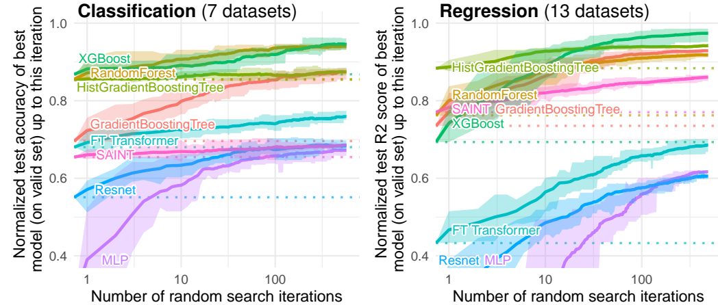
Figure 1: Benchmark on medium-sized datasets , top only numerical features; bottom: all features. Dotted lines correspond to the score of the default hyperparameters, which is also the first random search iteration. Each value corresponds to the test score of the best model (on the validation set) after a specific number of random search iterations, averaged on 15 shuffles of the random search order. The ribbon corresponds to minimum and maximum scores on these 15 shuffles.
