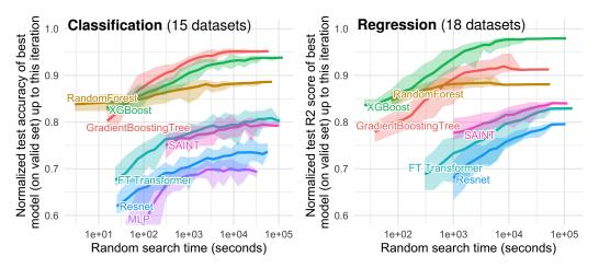
Figure 7: **Time benchmark on medium-sized datasets, with only numerical features**. The first random search iteration corresponds to default hyperparameters. Each value corresponds to the test score of the best model (on the validation set) after a specific time spent doing random search, averaged on 15 shuffles of the random search order. The ribbon corresponds to the minimum and maximum scores on these 15 shuffles.
