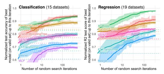
Figure 1: **Benchmark on medium-sized datasets, with only numerical features**. Dotted lines correspond to the score of the default hyperparameters, which is also the first random search iteration. Each value corresponds to the test score of the best model (on the validation set) after a specific number of random search iterations, averaged on 15 shuffles of the random search order. The ribbon corresponds to the minimum and maximum scores on these 15 shuffles.
