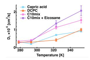
**Figure 4:** Global translational diffusion coefficient of all four samples as a function of temperature.
