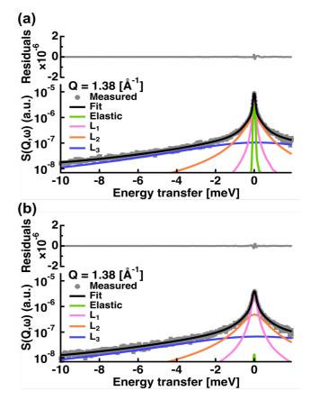
**Figure 2:** Examples of fit results for the spectra of (a) capric acid and (b) C10mix, both at  $Q = 1.38 \, \text{Å}^{-1}$  and  $T = 293 \, \text{K}$ . The grey circles are the data points with errors, the black line is the total fit line. The green line represents the elastic contribution convoluted by the resolution function. The magenta, orange and blue curves are the Lorentzian functions corresponding to slow, intermediate and fast motions, respectively, convoluted by the resolution.
