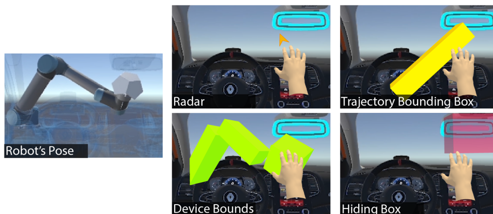
Figure 6. The bounds group. This group comprises techniques that bound the ETHD device for protecting the user from getting closer to the ETHD.
