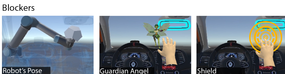
Figure 4. The blockers group. This group comprises techniques that interpose a virtual object between user and ETHD to block/avoid a possible unexpected collision.
