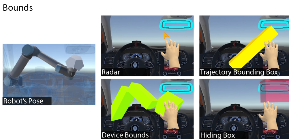
Figure 6. The bounds group. This group comprises techniques that bound the ETHD device for protecting the user from getting closer to the ETHD.
