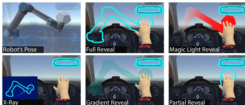
Figure 2. The revealers group. This group comprises techniques that display the ETHD's virtual counterpart in the virtual environment.
