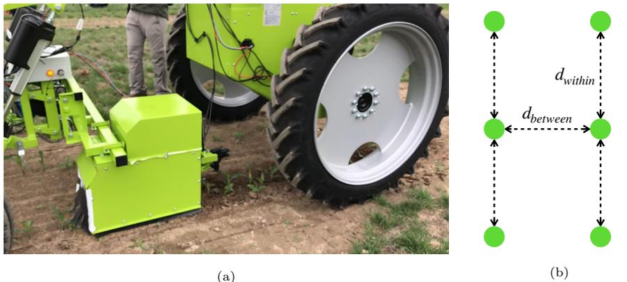
Figure 1: 1a: One BIPBIP weeding module embedded under an electric tractor operating on the left row of a maize bed in an experimental plot; 1b: Between-rows ( $d_{between}$ ) and within-row spacing ( $d_{within}$ ). Row direction is indicated by the arrow.
