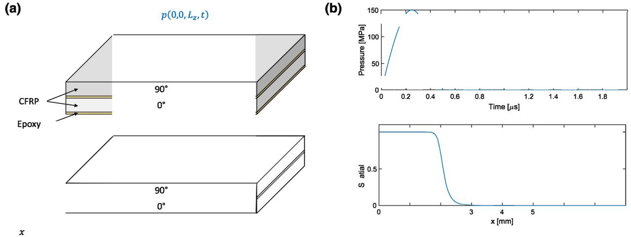
**Fig. 9** **a** Stacking configuration. CFRP plies thickness is  $140\mu\text{m}$  and Epoxy interplies thickness is  $30\mu\text{m}$ . **b** Time and spatial profiles of the applied loading
