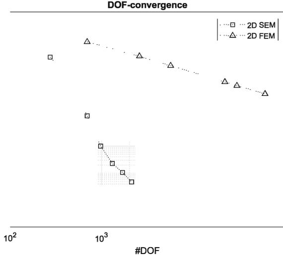
**Fig. 2** Error evolution obtained with 2D FEM and 2D SEM solvers with respect to a reference numerical solution computed with a grid of  $20 \times 10$  spectral elements of degree 10 (60,903 degrees of freedom)
