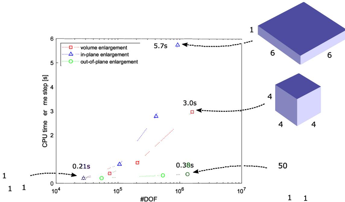
**Fig. 8** Evolution of the average CPU time per time step depending on the way of increasing the number of DOFs. Numbers next to the edges of the hexahedral domains indicate the scaling factors from the reference
