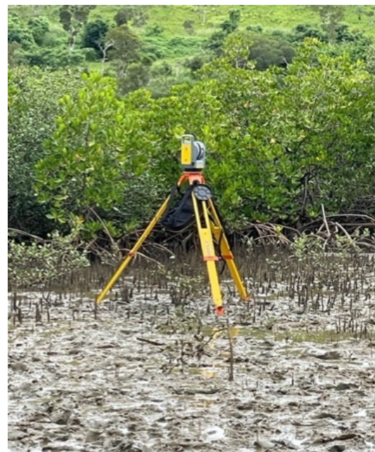
Figure 6. Laser scanning measurements using a TLS (Trimble X7).
