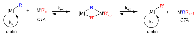
Scheme 2 General mechanism of coordinative chain transfer polymerization (CCTP) of olefins. M' is a main group metal or zinc
