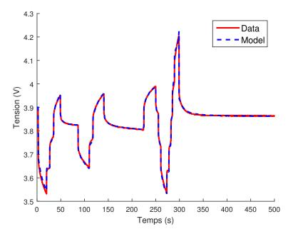
**Figure 9.** Voltage U(t) compared to the response  $U_2(t)$  of model in Figure 6 using the Volterra model (2) with kernel (27).
