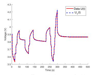
**Figure 7.** Voltage U(t) compared to the response of model in Figure 6 with the fractional transfer function (25).
