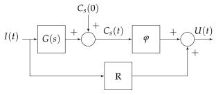
Figure 6. Model of a lithium-ion cell proposed in [38].
