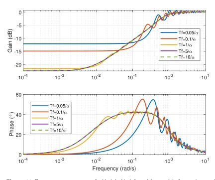
**Figure 11.** Frequency responses of  $x(j\omega)/u(j\omega)$  for  $\eta(t)=\eta_2(t)$ , for various values of  $T_f$ .
