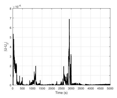
**Figure 10.** Error between voltage U(t) and the response  $U_2(t)$  of model in Figure 6 using the Volterra model (2) with kernel (27).
