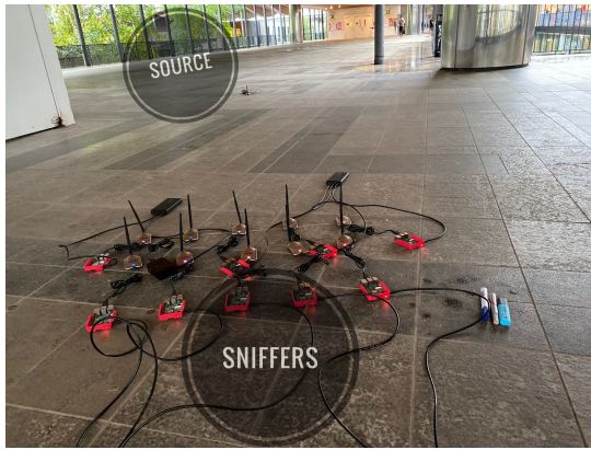
Fig. 1: Co-located sniffers and the source at a distance of 10m.
