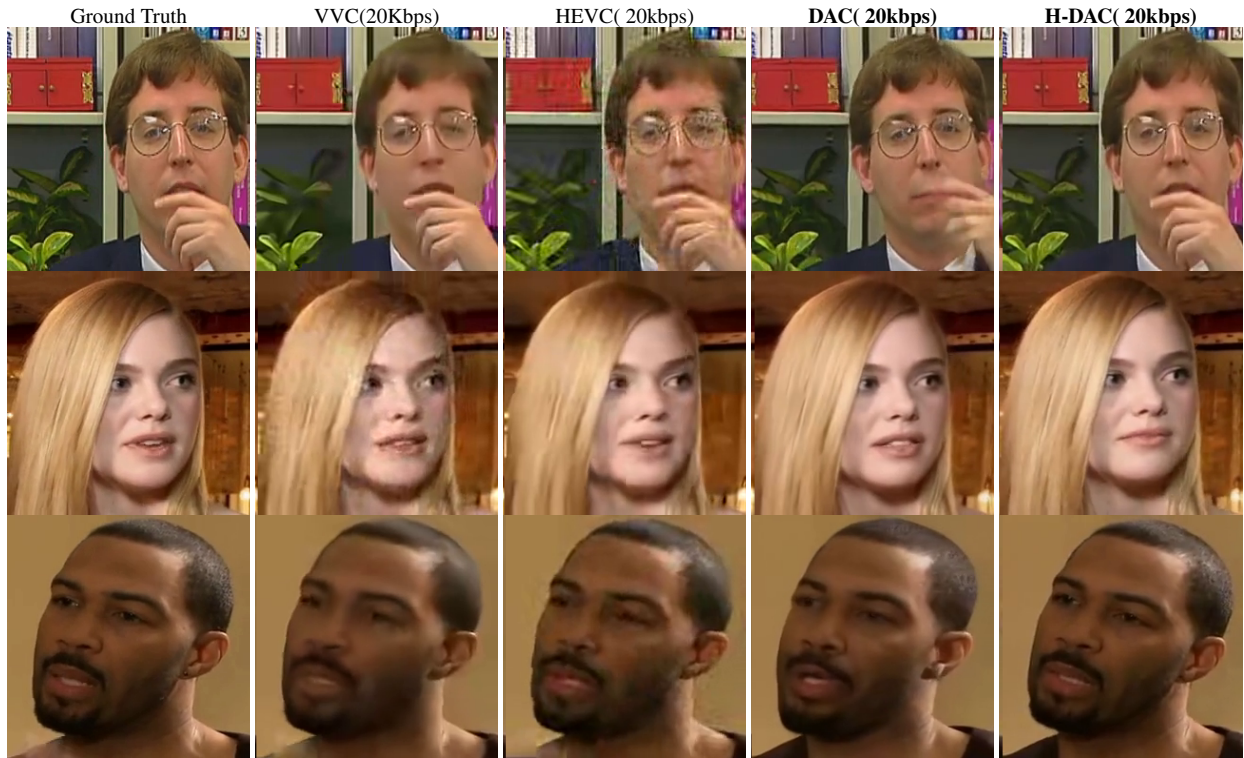
Fig. 2: Qualitative comparison of reconstructed images with our codec and state-of-the-art codecs at a similar bitrate. H-DAC significantly improves DAC in reproducing face expressions with good fidelity (e.g., the open mouth in the second row and the teeth in the third row), and is robust to non-face objects such as the hand in the first row. In addition, the synthesized images display lower distortion than HEVC and VVC.
