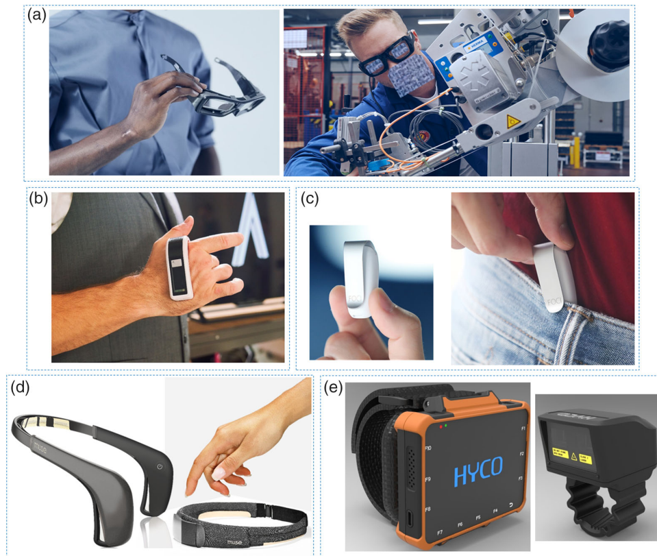
Figure 3. Examples of wearables for occupational productivity monitoring. a) ViewPoint Systems VPS 16 smart glasses have stereoscopic cameras that track spatial vision and have live streaming capabilities for mixed reality applications. b) Tactigon Skin uses sensors to detect hand gestures and AI to remotely interact with digital machines. c) The Tinylogic Foci clip-on device monitors the breathing patterns to estimate cognitive state of mind and suggests ways to avoid distraction at work. d) Muse 2 and Muse S headbands measure brain electrical activity and provide real-time feedback on body performance and mental focus. e) Hyco's W562 smartwatch enables hands-free barcode scanning for goods tracking and asset management. a) Reproduced with permission. [231] Copyright 2021, ViewPoint System; b) Reproduced with permission. [107] Copyright 2021, The Tactigon; c) Reproduced with permission. [121] Copyright 2021, Tinylogic Foci; d) Reproduced with permission. [114] Copyright 2021, Muse; and e) Reproduced with permission. [86] Copyright 2021, Hyco.
