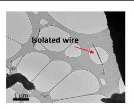
**Deposition on TEM carbon grid for TEM experiments**
