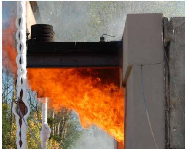
Figure 19. Flames through the opening (test n°1 – 17 min)
