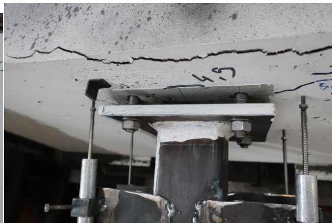
b) Slab reinforcement rupture
