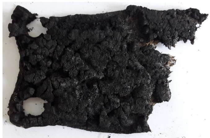
b) Test B1-2 : PVC surface in contact with the end-plate
