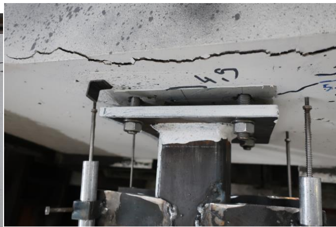
b) Slab reinforcement rupture
