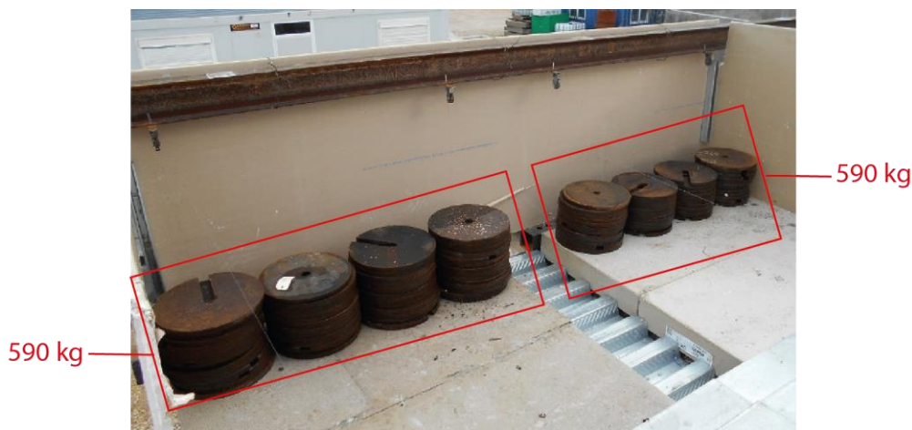
468 Figure 15. Load applied on the slab of balconies
