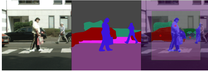
Fig. 8: Urban scene semantic segmentation example: input (left), coloured ground truth (centre), predicted segmentation (right). Model does not predict on crop boundaries, 3 circled pixels in the predicted area are subject to explanation.
