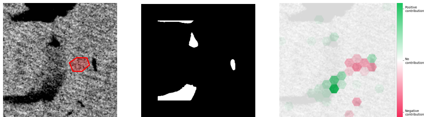
Fig. 1: An input Synthetic Aperture Radar image (left) is processed by a model for oil slick detection (centre). In order to explain prediction for a given region (red polygon on the left), the proposed SHAP based method provides a coloured map showing each image area’s contribution (right).
