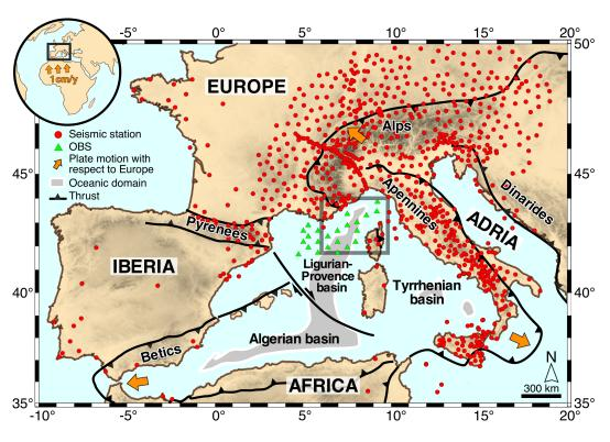
Figure 1. Tectonic map of the western Mediterranean region (modified from Faccenna et al., 2014; Jolivet et al., 2020) with locations of seismic stations used in this work (red circles: onshore sensors; green triangles: AASN OBS). The oceanic domains of the Ligurian-Provence, Algerian and Tyrrhenian back-arc basins are filled with gray color. The gray frame shows the location of the map in Figure 8a.
