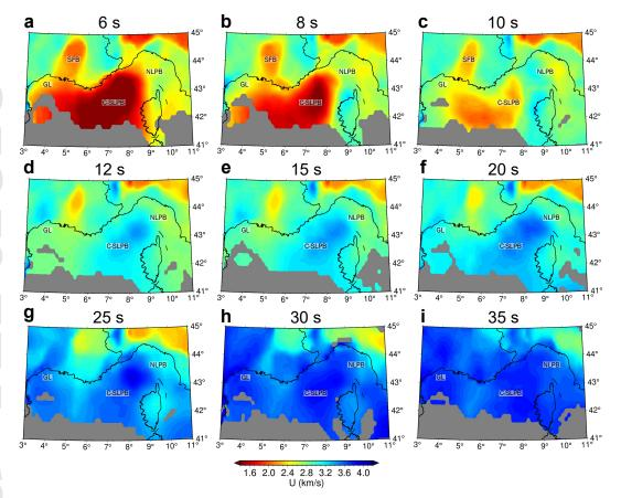
Figure 5. Group-velocity maps (average solutions) at 6 to 35 s periods, obtained with the Hierarchical Bayes reversible-jump algorithm. Only areas with uncertainty lower than  $0.5 \ km/s$  are shown. C-SLPB: central and southwestern parts of the basin, GL: Gulf of Lion, NLPB: northeastern Ligurian-Provence basin, SFB: southeast-France basin.
