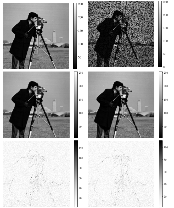
Fig. 2. Strong-scaling experiment results: ground truth and observations (first row), MMSE estimates (second row) and 95% credibility intervals (third row). For the rows 2 and 3, the results of the serial sampler [13] are reported on the left, those of the proposed approach on the right. Note that the credibility maps do not have the same scale to better highlight the distribution of uncertainties.
