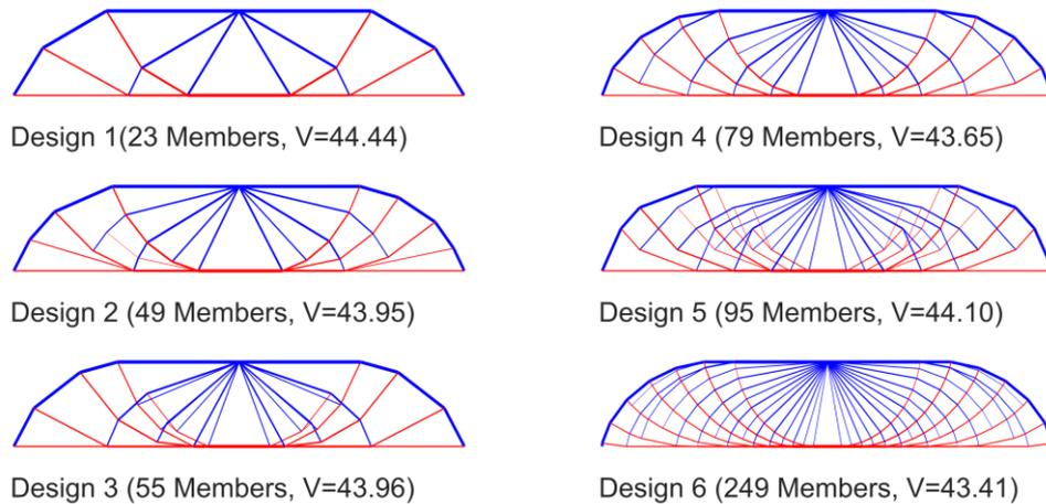
Figure 3 – “Equally” optimum truss designs of the MBB beam (the line thickness is proportional to the cross-sectional area).
