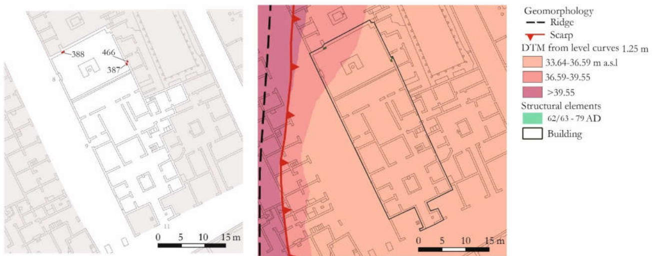
Figure 13. On the left is the plan of House of the Naviglio (VI 10, 8–10), with in red the structures built up with NYT elements. On the right the plan of the geomorphological evidence in the same area (elab. M. Covolan).
