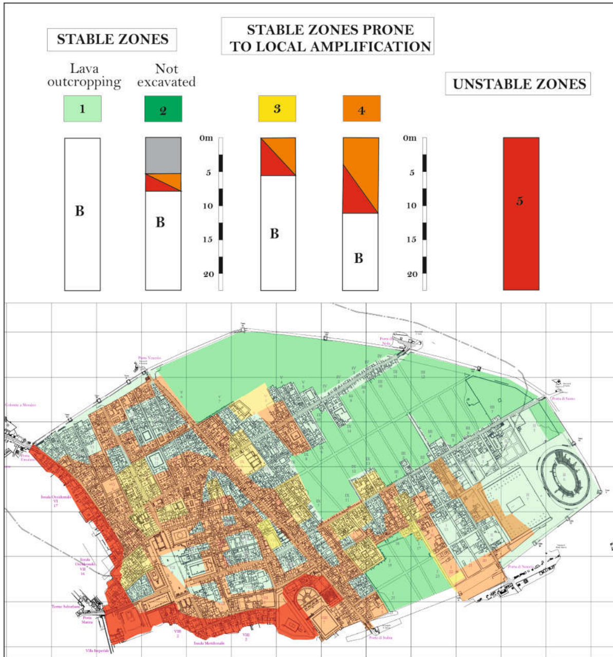
Figure 12. Seismic homogeneous microzones and seismic microzonation map of the Pompeii Archaeological Park.
