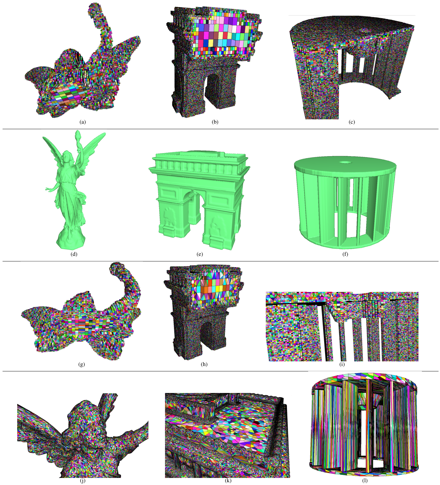
Fig. 18: Visual results of all methods applied to the three meshes used in the experiments in Section 7. First line: Hexahedra Subdivision; Second line: Marching-Cubes; Third line: Conformal Mesh; Fourth line: Mesh Transformation. Results for Marching-cubes are surfacic meshes; for other methods they are volumic meshes, drawn sometimes only partially to see the interior.
