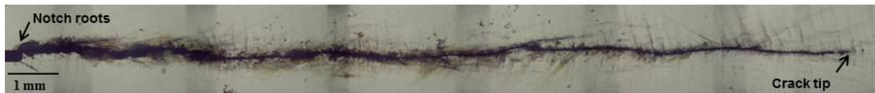
Figure 4 - Nearly-transverse secondary branches in mode II for 16NCD13 steel
