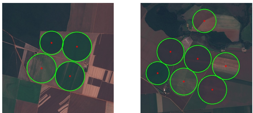
Figure 12. Examples of the location of center pivot irrigation systems using Hough transform.
