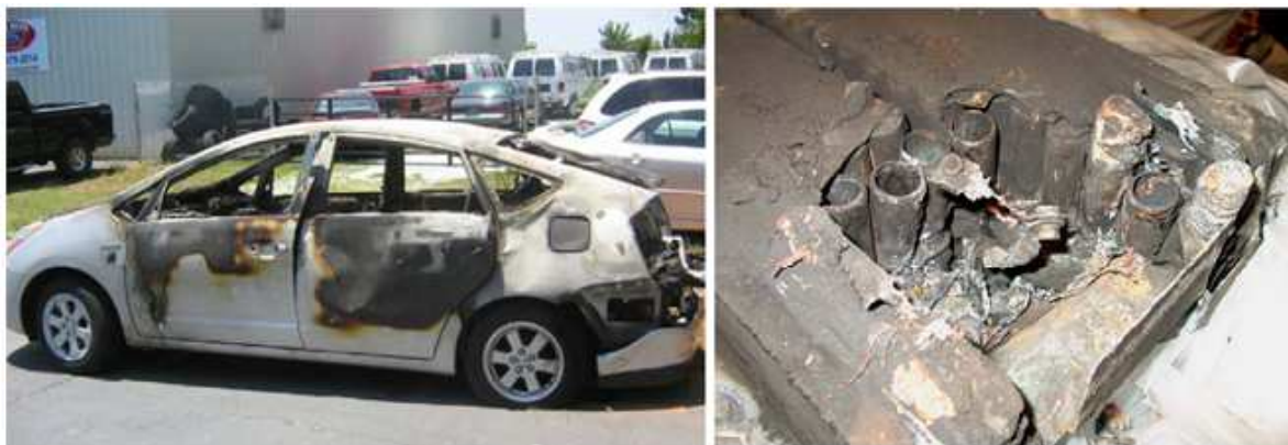
Fig. 4. EV and battery cells damaged by fire [49]
