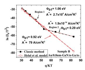
As can be seen, the Helal et al. model shows a homogeneous Schottky barrier height for both structures, since the  $ln(I_s/T^2)$  versus q/kT results in a linear dependence. Parameters  $\Phi_b$  and  $A^*$  were estimated at 0.84 eV and 98.43 A cm<sup>-2</sup>K<sup>-2</sup>, respectively for sample A and at 0.92 eV and 79 A cm<sup>-2</sup>K<sup>-2</sup> respectively for sample B.
