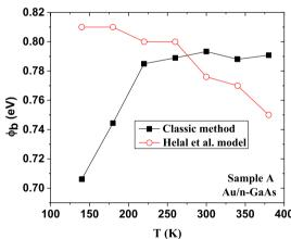
Figures 5 and 6 show the barrier height  $\Phi_b$  variation versus temperature for samples A and B, respectively.
