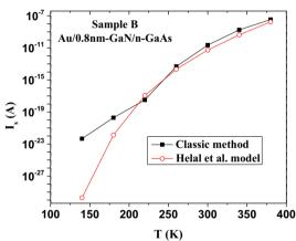
In addition, the  $\Phi_b$  extracted from the sample B is higher than of sample A. This is due to the presence of the thin GaN layer [45].
