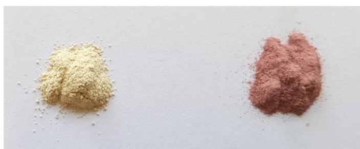
Figure 3: Ba 3 LiNb 2 O 8.5 □ 0.5 before and after the annealing at 1400°C in a sealed platinum tube showing the change in color, Beige-O 8.5 (left) and Pink-O 8.5 (right)
