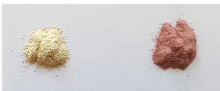
Figure 3: Ba 3 LiNb 2 O 8.5 □ 0.5 before and after the annealing at 1400°C in a sealed platinum tube showing the change in color, Beige-O 8.5 (left) and Pink-O 8.5 (right)
