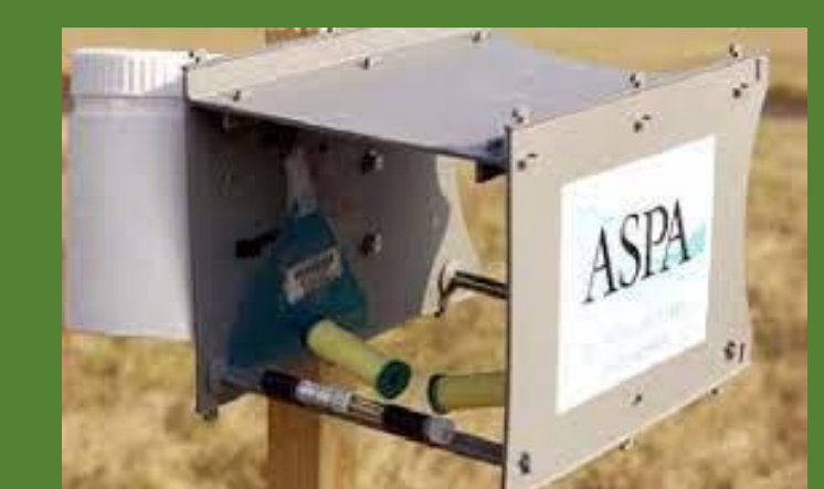
Figure 4 : Example of a passive tube device installed to measure benzene. Source : Atmo Grand Est
