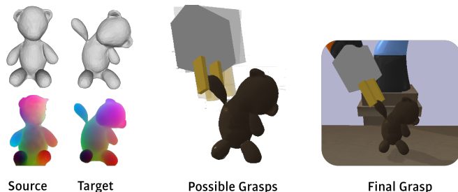
Fig. 1. Deformable object grasping by the proposed grasp transfer method. (left) Source and target meshes, and their functional maps. (middle) Transferred possible grasp configurations. (right) Executed best grasp.
