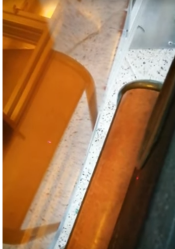
Figure 1. Laboratory characterization of the beamsplitter vibrations by creating a sound wave. The red laser pointing is visible in the center of the membrane. https://www.youtube.com/shorts/s95272u9b1Y
