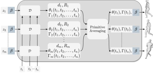
Figure 3. Implicit decoder. Given a sequence of latent primitives  $z_i$ , a body shape  $\beta$  and timestamps  $t_j$ , the decoder outputs a sequence of body meshes parameterized by  $\beta, \theta, \Gamma$ .  $z_i$  are decoded independently into segment parameters that include duration  $d_i$  and transformation  $R_i$ , and subsequently combined to decode a dense 4D motion.
