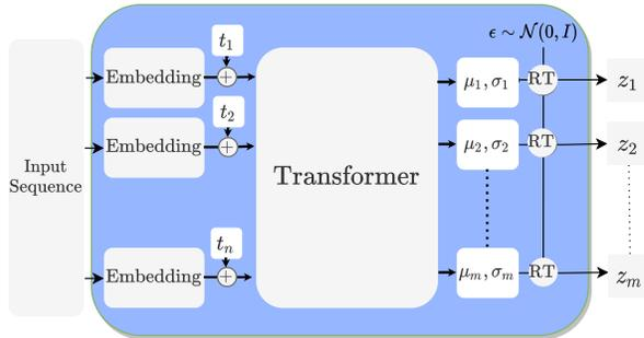
Figure 2. Encoder mapping an input sequence into a sequence of latent motion primitives  $z_1, \dots, z_m$ . The embedding is one multi layer perceptron for the parametric input and a PointNet [26] for point cloud input. Time stamps  $t_i$  are added as positional encoding. Transformer outputs a sequence latent distributions  $\mu_i, \sigma_i$  from which  $z_i$  are sampled using the reparametrization trick (RT).
