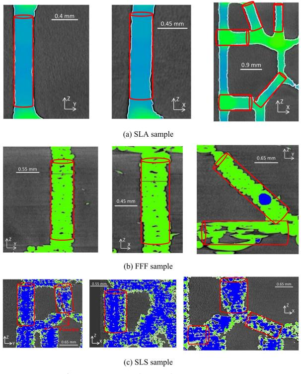
Figure 7. Strut cylindricity of sample 05 for the three processes.
