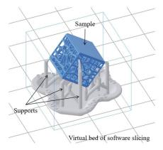
**Figure 2.** Orientation and supports needed for the SLA process.
