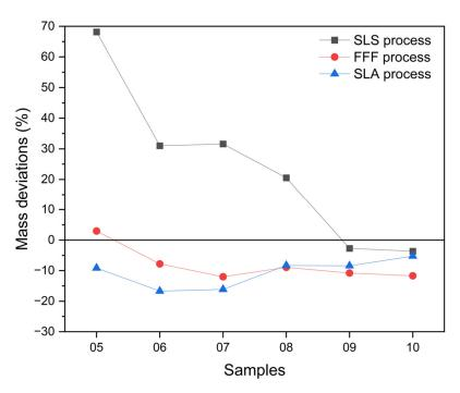
Figure 12. Mass deviations of the samples obtained with the three processes.
