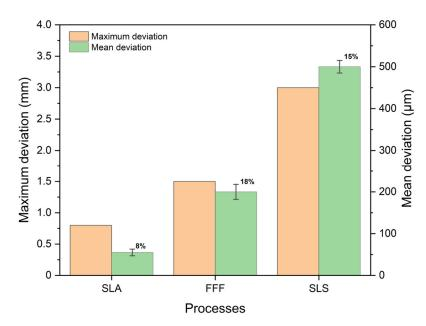
**Figure 6.** Dimensional deviations of the printed sample 05 from the CAD model.
