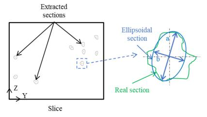
**Figure 9.** Principle of the statistical analysis of the eccentricity of cross-sections.
