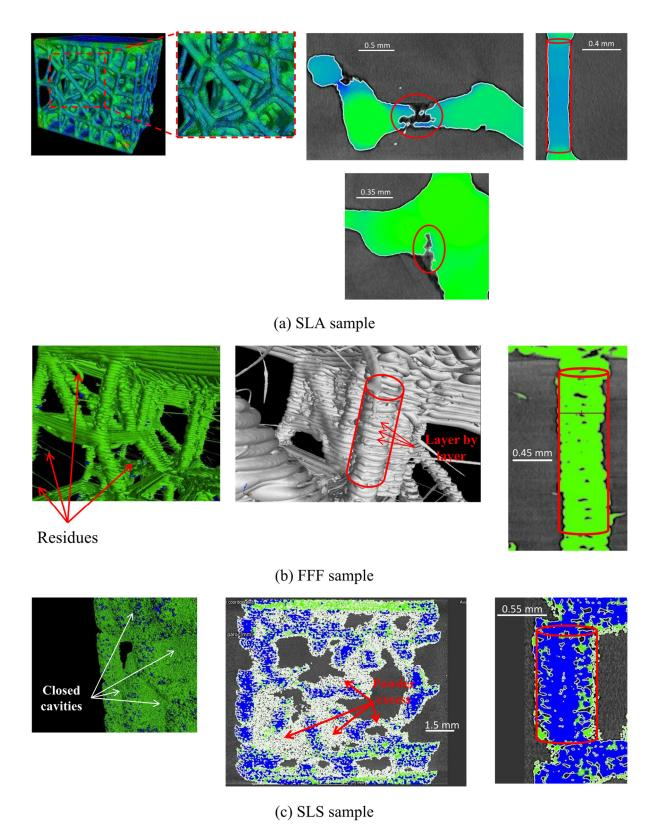
**Figure 5.** Tomography observations of the quality of samples from 05 to 10.
