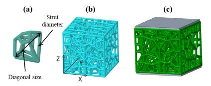
**Figure 1.** Steps for the architected structure generation: (a) basic pattern, (b) architected structure, (c) addition of plates on the top and bottom faces.
