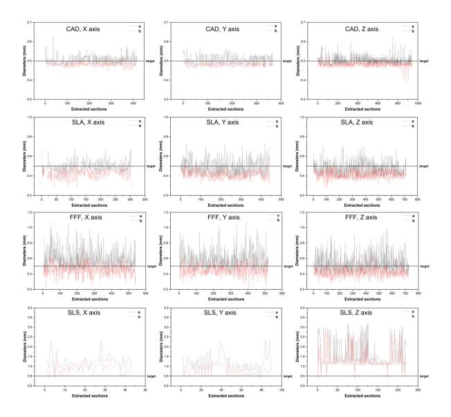
**Figure 11.** Representation of the diameters a and b, sample 05 for CAD model and the three processes.
