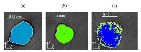
Figure 8. Examples of sample 05 strut sections (a) SLA, (b) FFF, (c) SLS.
