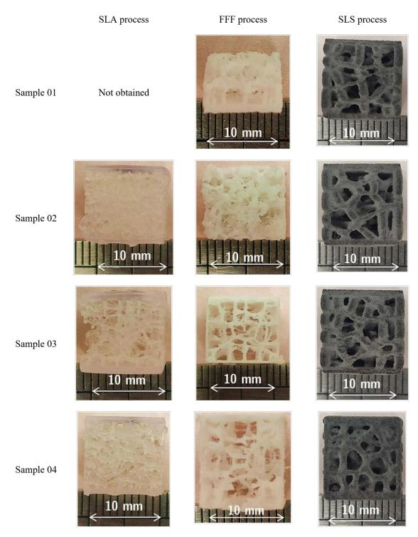
$\textbf{Figure 3.} \ \ \text{Defects in samples with strut diameters lower than } 0.5 \ \text{mm}.$
