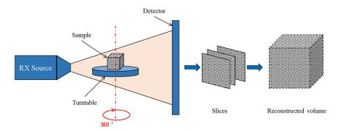
Figure 4. X-ray tomography principle.
