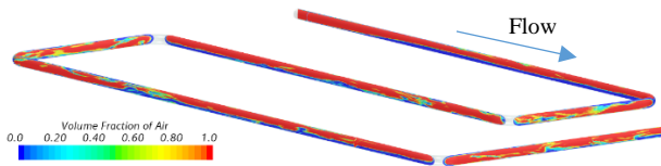
Figure 5. Snapshot of CFD predicted contours of gas volume fraction (case 1) without inlet Y-piece
