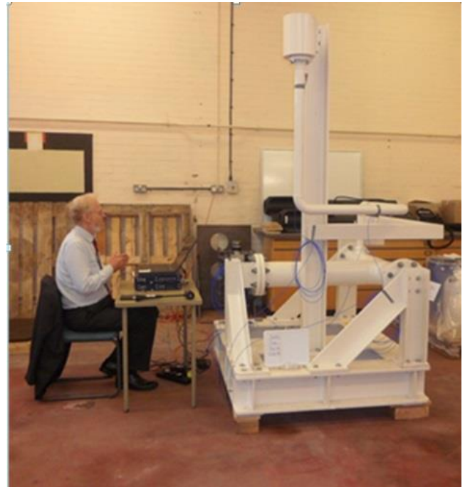
Figure 9. A full-scale pipework system that was tested in air and also in water.
