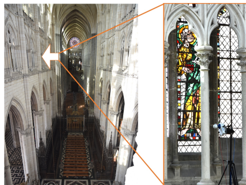
Fig. 1: Inside Amiens Cathedral, France: (left) 42m height at the center; (right) stained-glass III scanned by a hyperspectral head in the triforium , a corridor at 20m above the ground.
