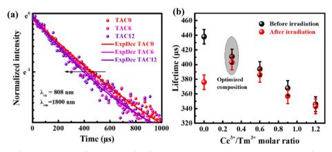
**Fig. 3.** (a) Decay curves of the  ${}^{3}F_{4}$  excited state of Tm<sup>3+</sup> ions from the  ${}^{3}F_{4} \rightarrow {}^{3}H_{6}$  emission transition (1800 nm) under pumping into  ${}^{3}H_{4}$  (808 nm) in the TAC glasses with different Ce<sup>3+</sup>/Tm<sup>3+</sup> ratios before irradiation. (b)  ${}^{3}F_{4}$  excited state lifetime values of Tm<sup>3+</sup> before and after 100 kGy irradiation as a function of the Ce<sup>3+</sup>/Tm<sup>3+</sup> molar ratio.
