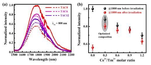
Fig. 2. (a) Fluorescence spectra of the TAC alumino-silicate glasses before (solid curve) and after (dash curve) 100 kGy  $\gamma$ -ray irradiation measured under excitation of  $\lambda_{ex} = 808$  nm aser diode; (b) The luminescence intensity of the Tm<sup>3+</sup> ion at approximately 1800 nm as a function of the Ce<sup>3+</sup>/Tm<sup>3+</sup> molar ratio.
