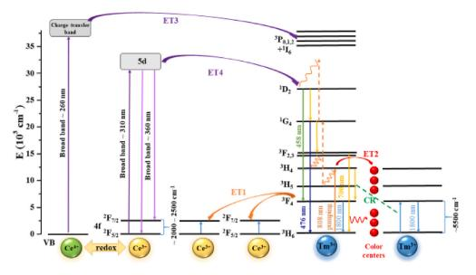
Fig. 8. Schematic diagram of energy transfer mechanisms after excitation into the high-energy side. ET: Energy transfer.
