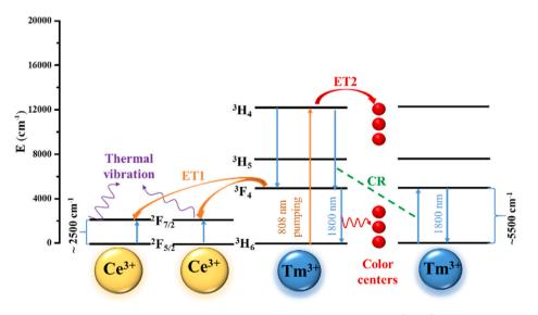
**Fig. 5.** Schematic diagram of the energy transfer mechanism limited to the near IR spectral range among  $Tm^{3+}$ ,  $Ce^{3+}$  and color centers. ET: energy transfer, CR: cross-relaxation. (For interpretation of the references to color in this figure legend, the reader is referred to the Web version of this article.)
