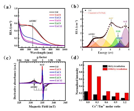
Fig. 4. (a) RIA spectrum of the TAC glasses, (b) Gaussian decomposition of the RIA spectrum of the 1Al glass, (c) EPR spectra (300 K) of 1 kGy  $\gamma$ -ray irradiated TAC glasses, (d) normalized double integration intensity of defects as a function of the Ce<sup>3+</sup>/Tm<sup>3+</sup> molar ratio.
