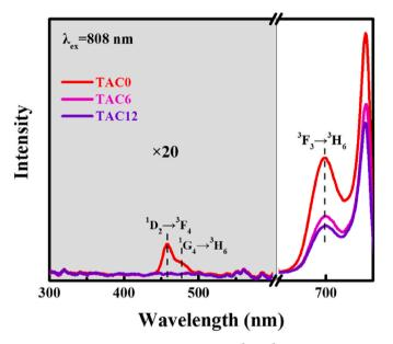
Fig. 7. Up-conversion emission spectra of  $Ce^{3+}/Tm^{3+}$ -co-doped aluminosilicate glasses, measured under excitation of  $Tm^{3+}$  at  $\lambda_{ex}=808$  nm of laser diode.
