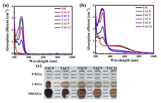
**Fig. 1.** Absorption spectra of the TAC alumino-silicate glasses (a) before and (b) after 1 kGy γ-ray irradiation. (c)Photography of the TAC alumino-silicate glasses before and after irradiation.
