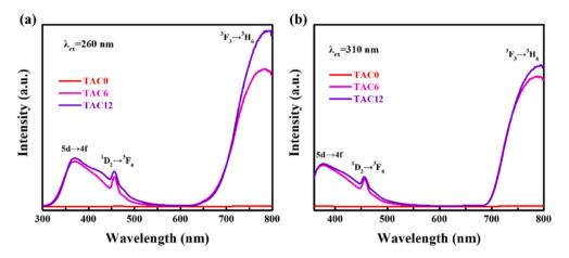
**Fig. 6.** Emission spectra of TAC0, TAC6 and TAC12 samples into UV radiations at both 260 nm (Ce<sup>4+</sup> ions) and 310 nm (Ce<sup>3+</sup> ions) at RT. We observe a Ce<sup>3+</sup> 5d $\rightarrow$ 4f broad band and some lines of Tm<sup>3+</sup> ions, including  ${}^{1}D_{2}\rightarrow{}^{3}F_{4}$  at 458 nm and  ${}^{3}F_{3}\rightarrow{}^{3}H_{6}$  between 700 and 800 nm.
